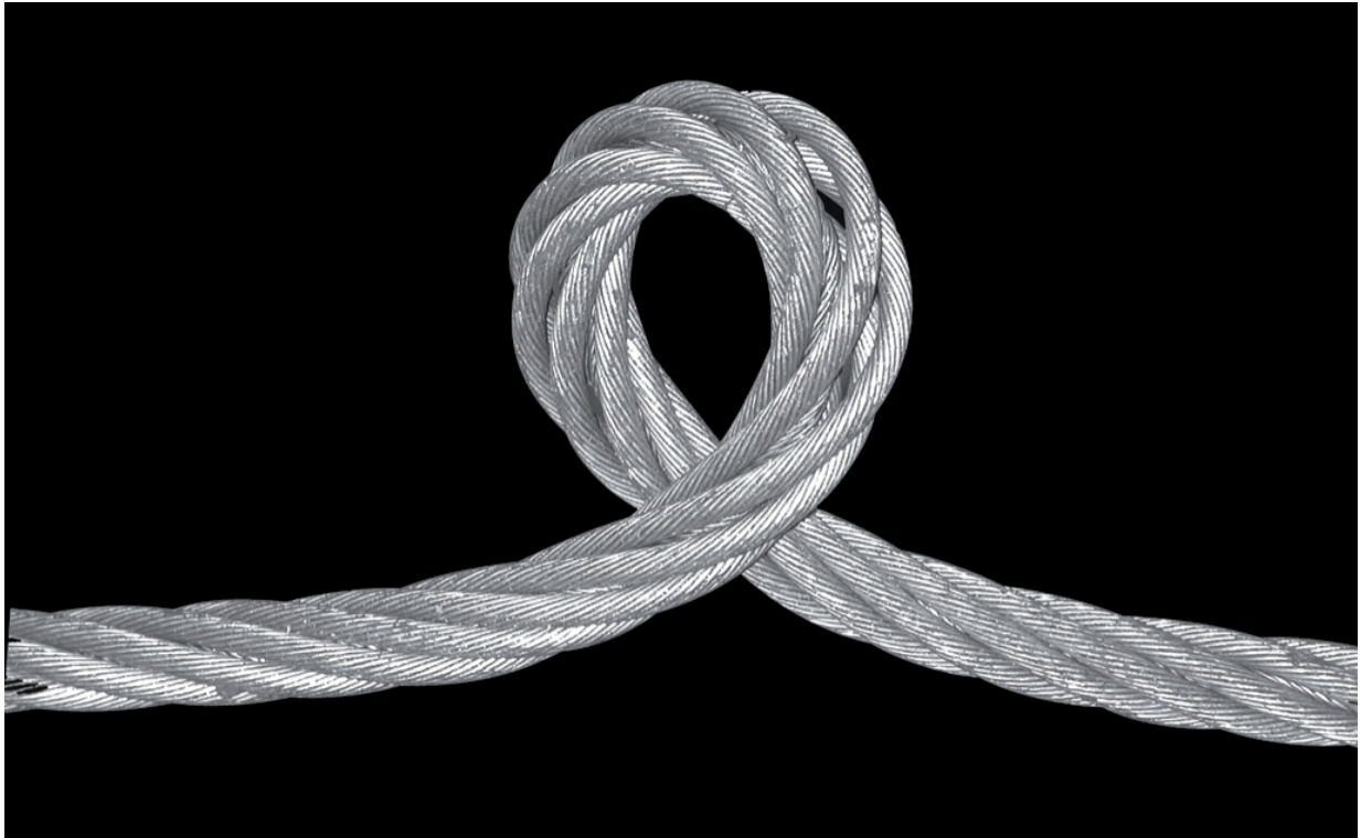
Fig. 21: A kink in a wire rope which is apparent at low tension.
