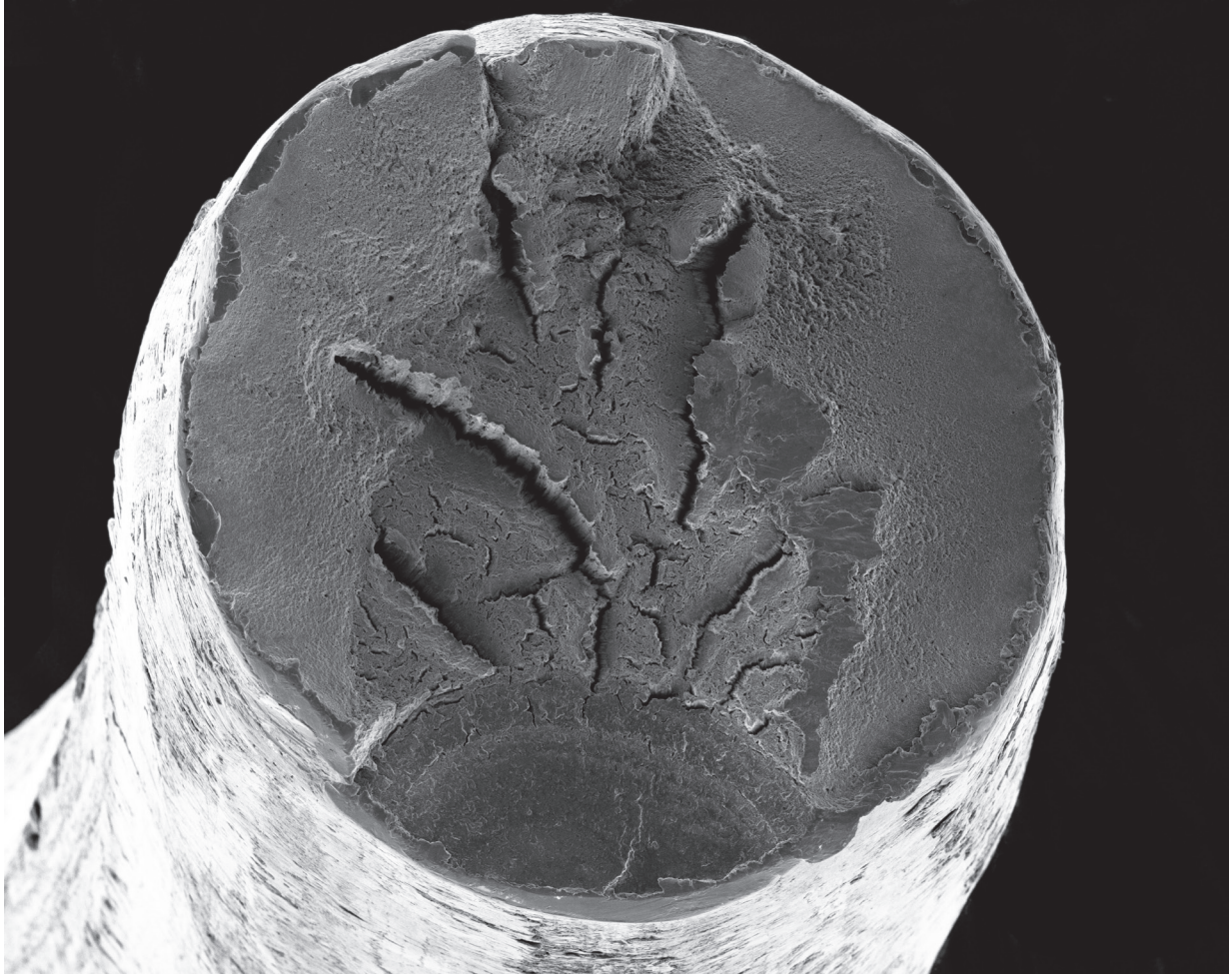
Fig. 10: Typical outer wire break surface from a rope which had “jumped the sheave” (scanning electron microscope photograph by the author).
