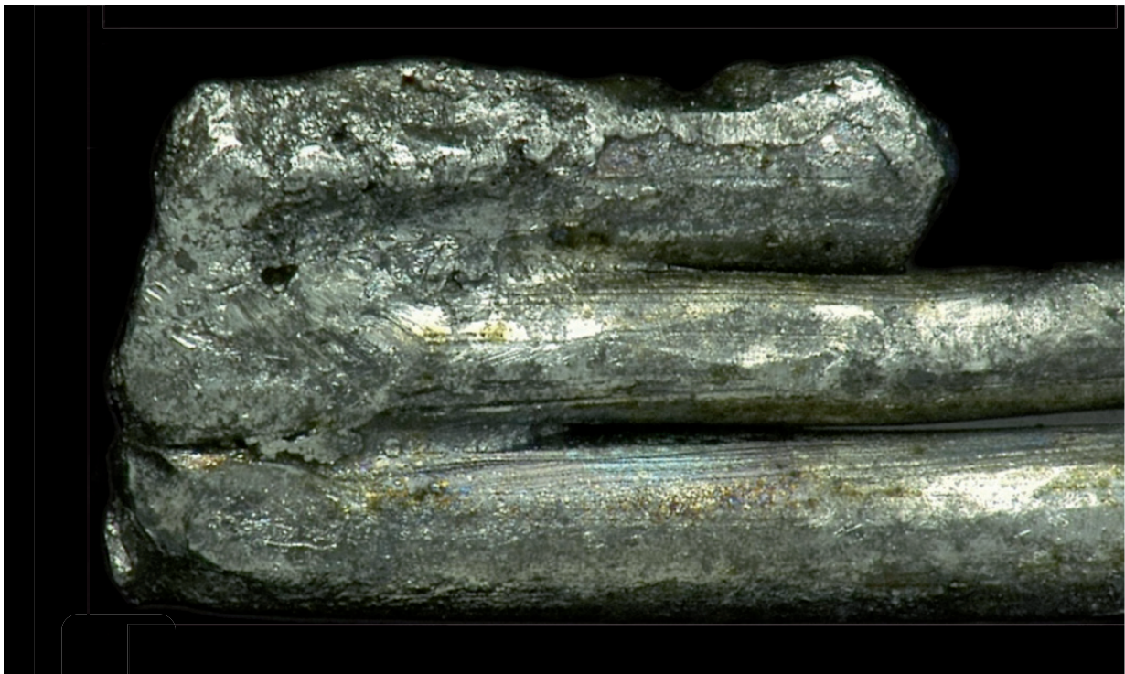
Fig. 12: Individual rope wires welded together as a result of lightning strike discharge through the rope.
