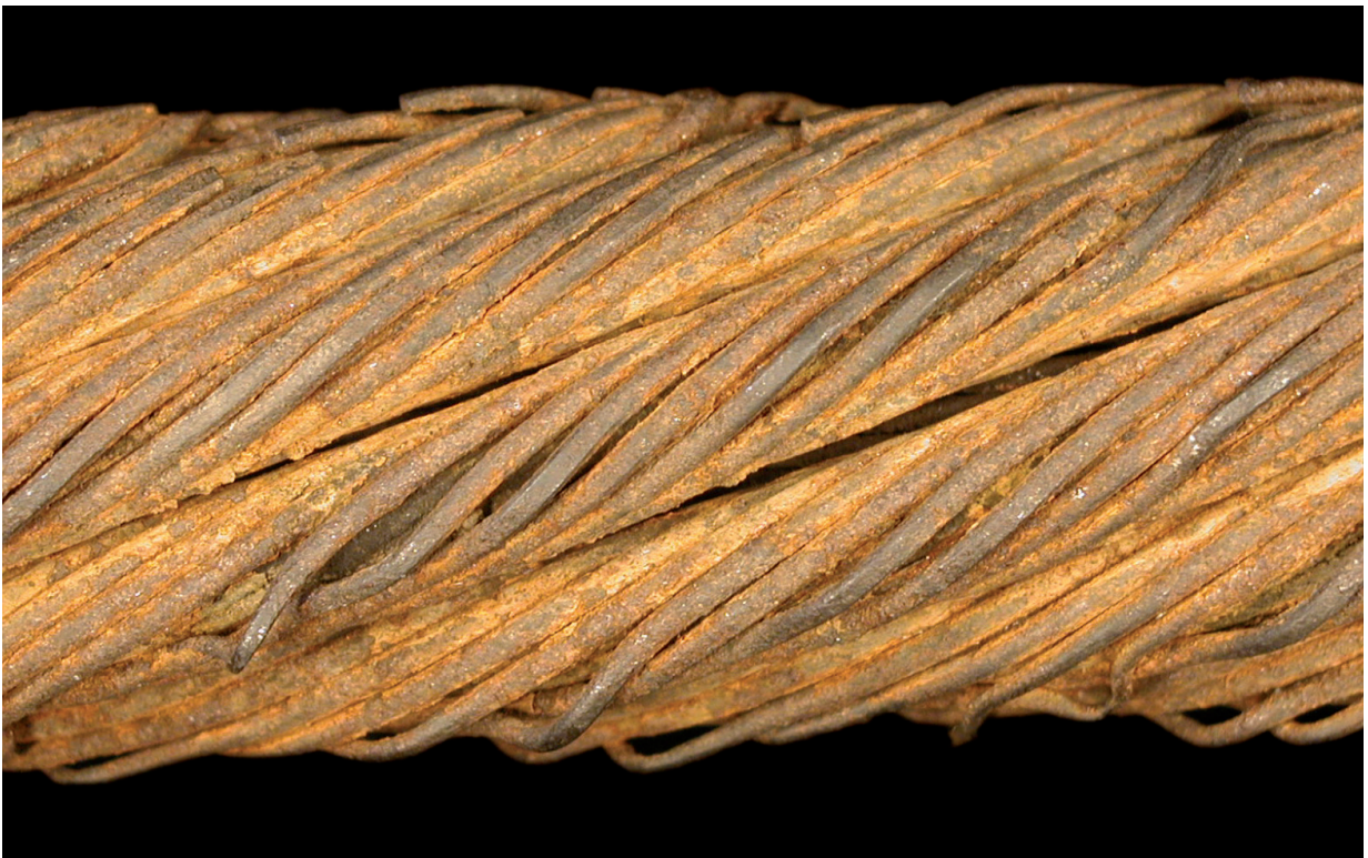
Fig. 16: A wire rope in which the wires have become too hot and annealed.
